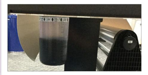
The unit's waste ink tank is easily removable, requiring the operator to simply unscrew it from the bottom of the printer, empty and replace. Users will be prompted with an "empty drain bottle" control panel message.
