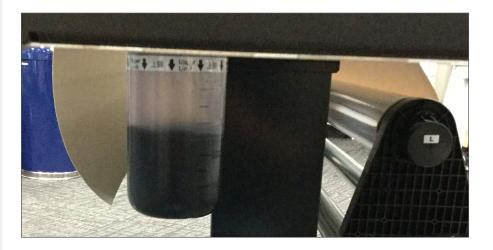
The unit's waste ink tank is easily removable, requiring the operator to simply unscrew it from the bottom of the printer, empty and replace it. Users will be prompted with an "empty drain bottle" control panel message.
