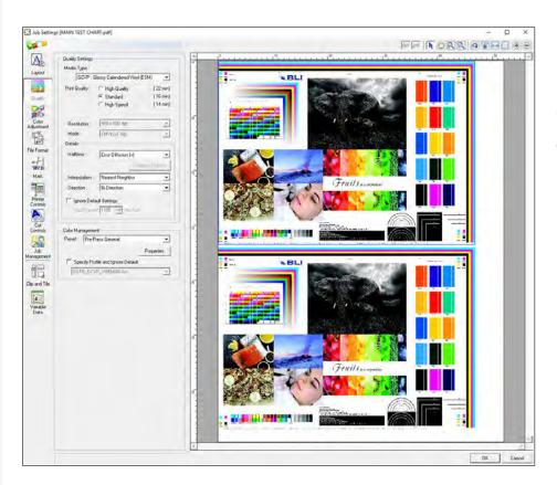
Detailed settings – layout, quality, color adjustment, file format, mark, printer controls, cut controls, job management, clip and tile, and variable data – can be applied in the clearly labeled tabs by clicking on a specific job in the VersaWorks Job List.
