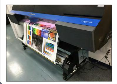
The take-up system, which is optional with the TrueVIS VG-640, enables multiple jobs to be readily collected onto a core facilitating unattended print runs.
