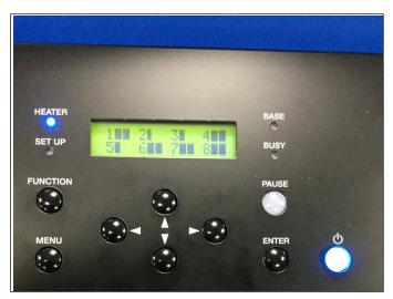
The ink indicator on the control panel displays one or two bars for the remaining ink level and lists numbers for each color instead of the actual color. It is presented in this manner because ink colors can be positioned in different slots on the device, depending on its ink color configuration.
