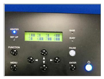
The ink indicator on the control panel displays one or two bars for the remaining ink level and lists numbers for each color instead of the actual color.
