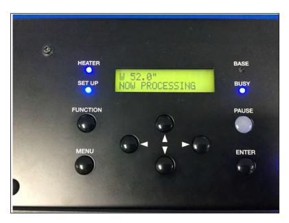
The unit's control panel is basic and features two lines of text and nine buttons. Common selections for media advance and cut, printhead cleaning, nozzle check, and heater adjustments are located several layers deep in control panel sub-menus. While printing, the panel displays the media width and print status.
