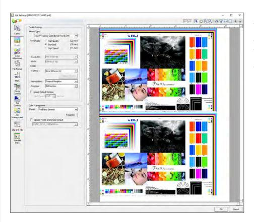
Detailed settings – layout, quality, color adjustment, file format, mark, printer controls, cut controls, job management, clip and tile and variable data – can be applied in the RIP's clearly labeled tabs by clicking on a specific job in the VersaWorks Job List.
